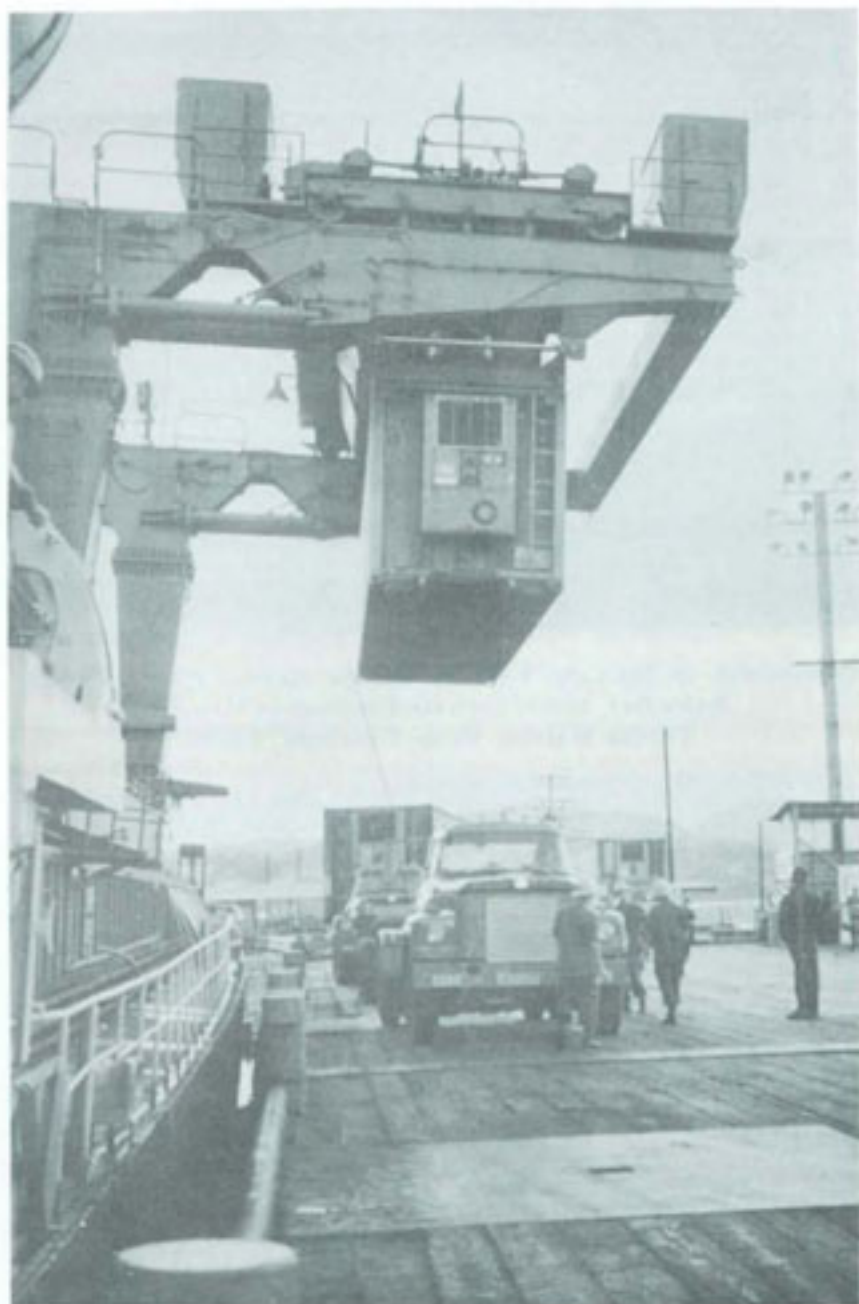
UNLOADING OF SEA-LAND VANS BY CRANE OF CARGO SHIP AT CAM RANH BAY
